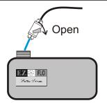
Step 5 - Fill tank with water until the tank overflows by opening the shut off valve.
